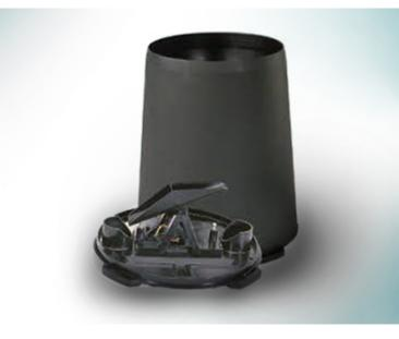
The IRG02, is a tipping-bucket rain gage. It measures rainfall in 0.01 in. increments. The IRG02 funnels precipitation into a bucket mechanism that tips when filled to its calibrated level. A magnet attached to the tipping mechanism actuates a switch as the bucket tips. The momentary switch closure is counted by the pulse-counting circuitry of our data loggers.
